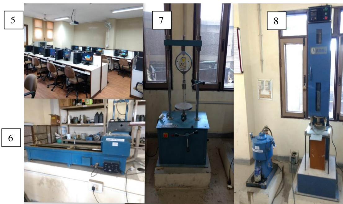
5. Civil Engineering Software Lab 6. Ductility Apparatus 7. CBR Testing Machine 8. Bitumen Extractor/ Marshall Mould Sampler
