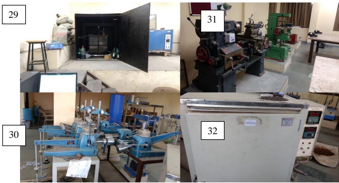
29. Biodegradation Settlement Analyzer 30. Consolidation Apparatus
