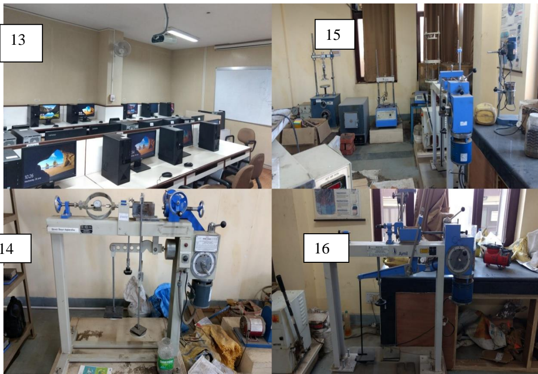
13. Civil Engineering Software Lab 14. Direct Shear Test Apparatus 15. Triaxial Shear Test Apparatus 16. Unconfined Compression Machine
