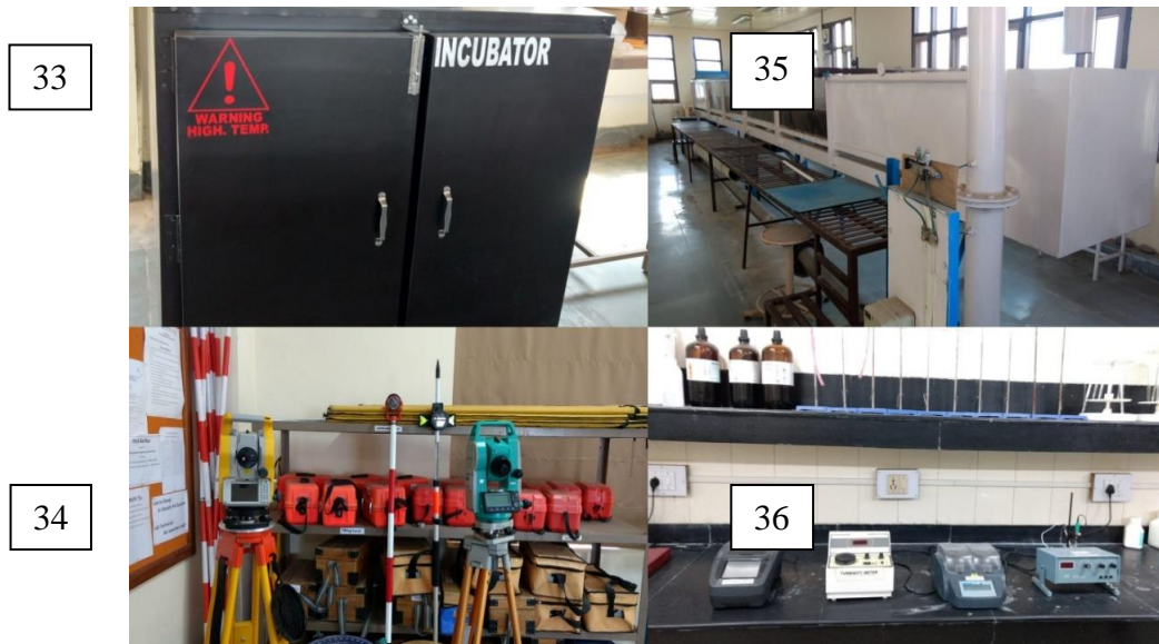
33. Biogas Incubator 34. Total Station/ Theodolite/ Auto Level/ Dumpy Level 35. Open Channel Flume 36. COD Digester/ pH Meter/ Conductivity Meter/ Turbidity Meter
