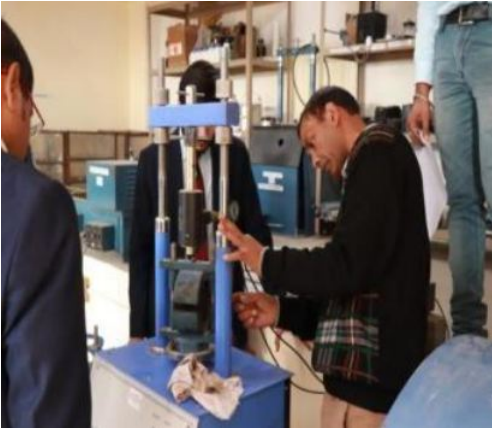
Marshal stability test (Highway Engineering lab)
